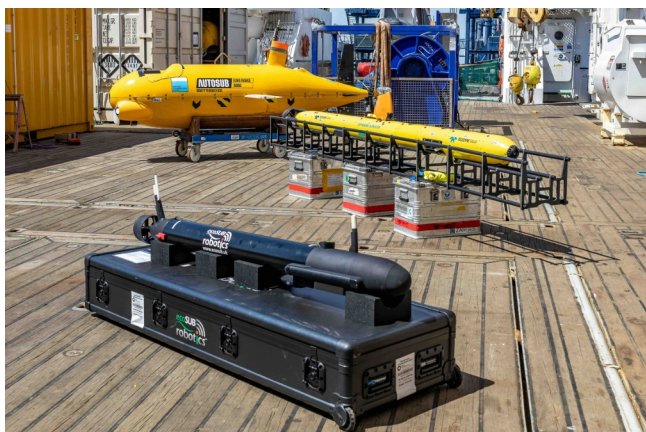
AUVs on the aft deck of the RRS Sir David Attenborough ahead of its GIANT mission. Pictured are Autosub Long Range, a Teledyne Gavia and an ecoSUB Robotics AUV. Photo from Sonardyne.
