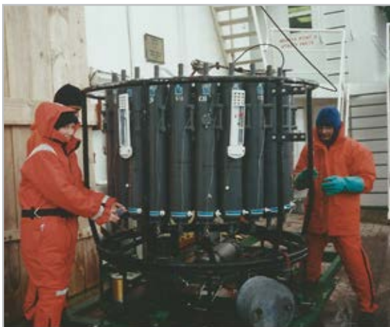
The RRS Discovery CTD rosette then and now Left Discovery III cruise D200 in 1993. (Photo: John Gould) Right Discovery IV cruise DY078 in 2017. (Photo: Penny Holliday)
