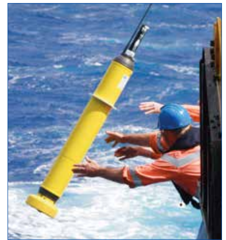
Launching an Argo float from Australia's RV Southern Surveyor. (Photo: Alicia Navidad, CSIRO)
