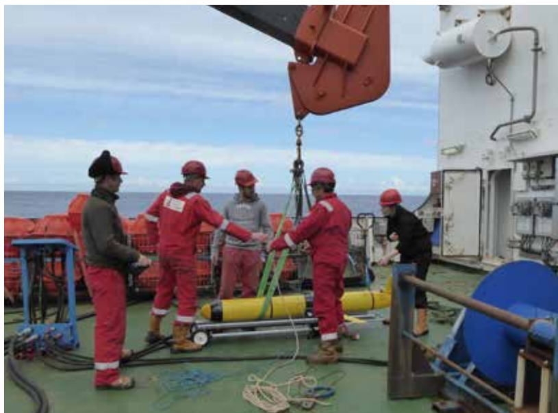
Figure 4 Preparing to deploy an autonomous underwater glider from a research ship. (By courtesy of the National Oceanography Centre)
