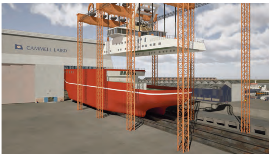
Right Artist's impression showing how the RRS Sir David Attenborough superstructure (decks 7 to 12) will be placed on to the main body of the vessel at the Cammell Laird shipyard in Birkenhead (© Roll Royce)
