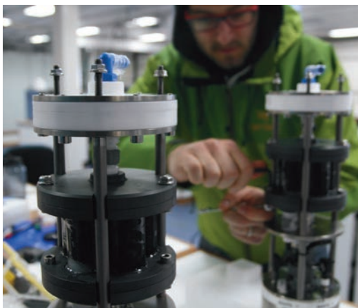
Figure 6 The author preparing Miniature Autonomous Pumps (MAPs) for their first sea-going trial during NERC's Shelf Seas Biogeochemistry Programme aboard the RRS Discovery. MAPs pumped measured volumes of ocean bottom waters through in-line particle filtration and radioisotope sampling apparatus with a view to measuring vertical gradients of chemical properties that could be used to derive fluxes across the benthic boundary layer. The MAPs were designed and built in collaboration with NOCS in Southampton. (Photo by courtesy of Torben Stichel)
