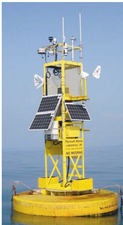
Figure 3 Upper L4 buoy on station showing the atmospheric instrument array around the top ring, including solar irradiance, wind speed and meteorological sensors as well as communication aerials. Wind generators and solar panels are clearly seen, along with the instrument control boxes just above the 'No Mooring' sign. Battery boxes are situated just above the surface of the 3.1 m diameter float.
