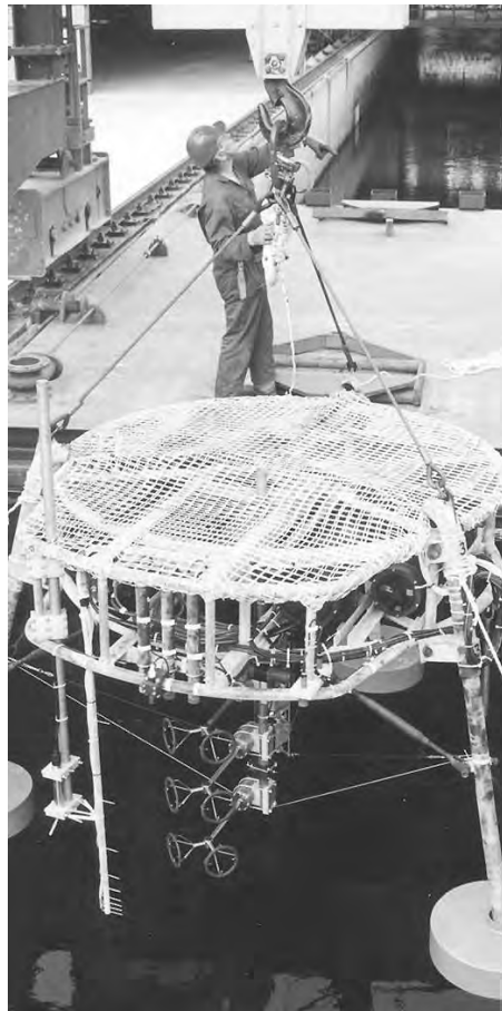
Figure 5 (a) Photograph of the Delta flume showing the wave generator at the far end of the flume and, in the centre, the sand bed used in the study. (b) STABLE II, the instrumented tripod, developed at the Proudman Oceanographic Laboratory by colleague John Humphery, being placed onto the sand bed. (c) Waves produced for the study travelling away from the wave generator at the far end.
