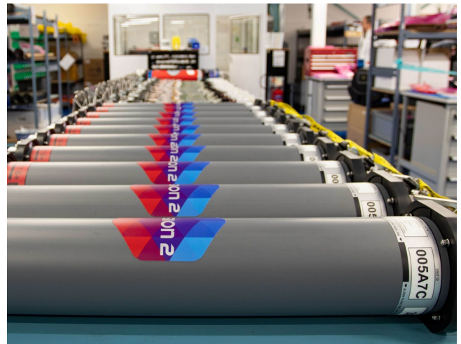
NOR's investment includes several Sonardyne Compatt 6+ LBL and USBL transponders. This image shows Compatt 6+ units being manufactured at Sonardyne's Headquarters in Hampshire, UK.
