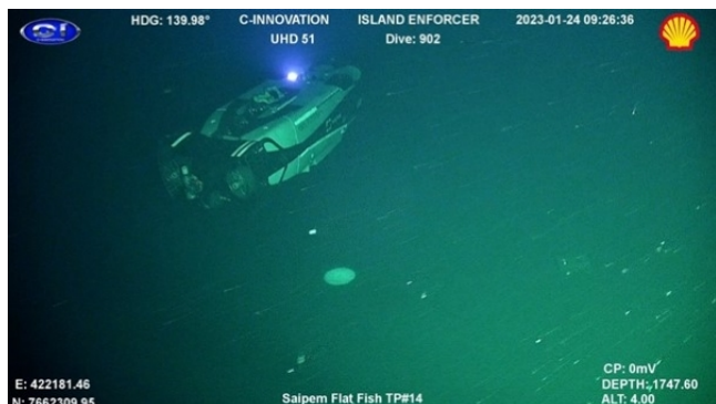
Field test image of the Saipem FlatFish placed above the OD OBN harvesting data using optical communications.
