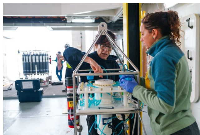
WHOI's Maria Pachiadaki and Lizt Osorio Pando prepare the Microbial Sampler for deployment. (Photo by: Alex Ingle, Schmidt Ocean Institute)
