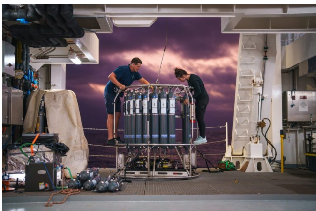
Josh O'Brien and Annabelle Adams-Beyea remove Niskin bottles from the CTD rosette prior to a re-deployment. Highly sensitive oxygen sensors were mounted on the CTD rosette which were used to make measurements of the extent of the oxygen minimum zone. (Photo by: Alex Ingle, Schmidt Ocean Institute)
