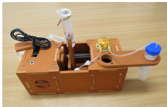
The "PlanktoScope", an ultra-low-cost microscopic imaging device
