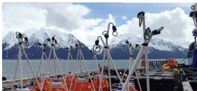
Sonardyne's Fetch long-life subsea sensor logging nodes enable subsea to surface data acquisition over periods of up to 10 years.
