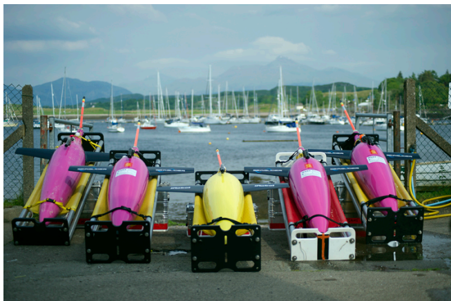
Ocean-going gliders can collect data for months at a time in some of the most remote parts of the ocean
