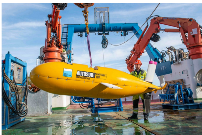
NOC's Autosub Long Range (ALR) autonomous underwater vehicle (AUV). Photo from NOC.
